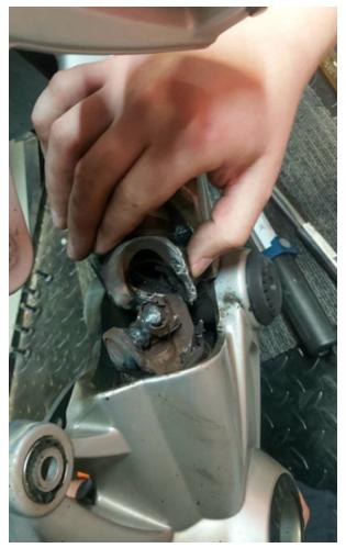
That doesn't look good. This is NOT a cause of spline lubrication or unheard of in Rxxxx motorcycles. Mine was at 136 000km.
